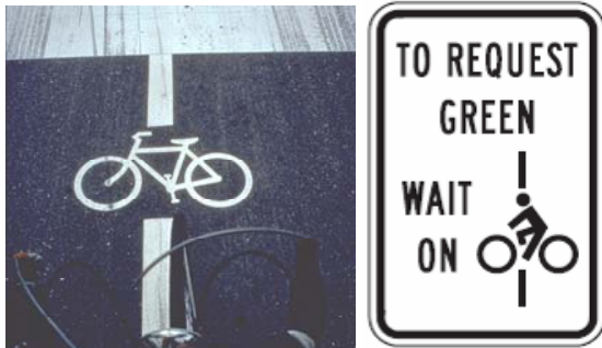
Figure 8. Signal activation marking and sign.
